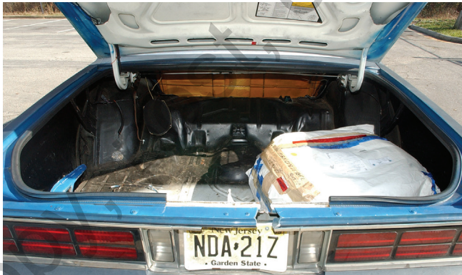
PHOTO 1.2 Notice how the trunk of the vehicle was configured so that a person could lie in it. Also observe the notch cut out of the trim to accommodate the barrel of a rifle.
