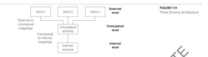
In the mid-1970s, the concept of data independence led to the proposal of the Three Schema Architecture depicted in Figure 1.11. The word **schema** as applied to databases means database description. The Three Schema Architecture includes three levels of database description. The <u>external</u> level is the user level. Each group of users can have a separate external view (or view for short) of a database tailored to the group's specific needs.
